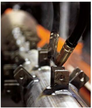
With the ABB robot, Kverneland now have one process, compared with four in terms of welding the rotor.
