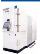
This Sinox CemeCon setup allows Lars Pleth Nielsen and his team to deposit coating materials that give substrates required properties such as hardness, conductivity and friction. It is also being used for research on self-cleaning surfaces and surfaces for solid oxide fuel cells.
